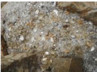
Shell lime mortar, Spiky Bridge
